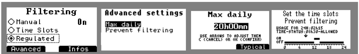
Figure 5. Filtering programming screens in regulated mode
