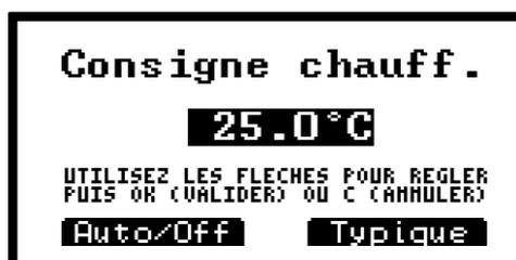
Figure 14. Heating target value setting screen
