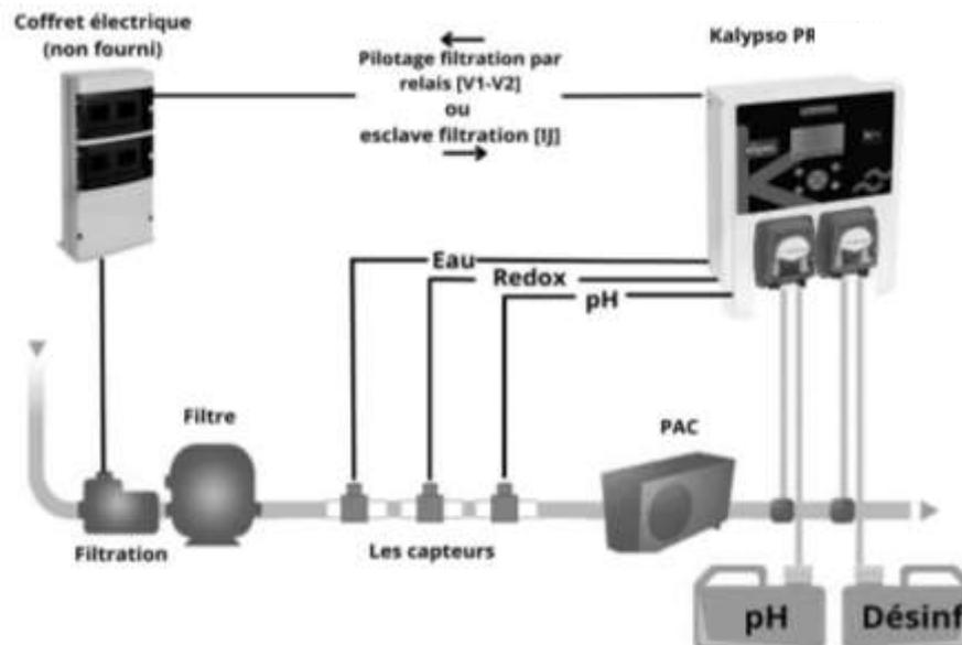
Figure 8. *Installation Kalypso PRO*
